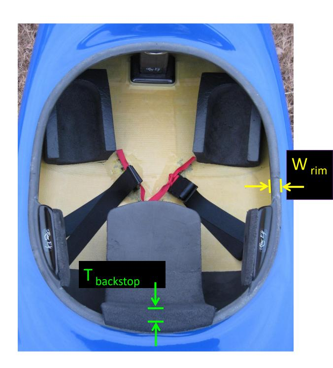
T backstop = thickness of backstop (don't include rim)
